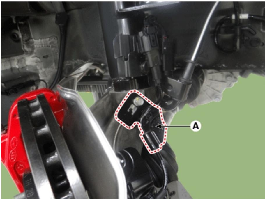
6. Disconnect the ECS connector (A) and then remove the wheel speed sensor bracket.
