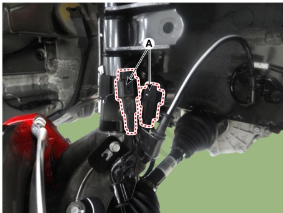
7. Remove the bracket (A) and then disconnect the connector (B).
